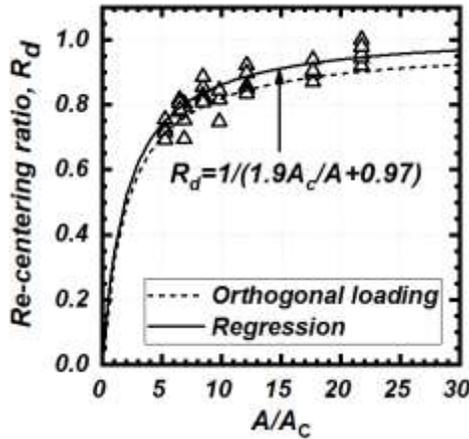
Figure 6. Effect of  $A/A_c$  on re-centering ratio.
