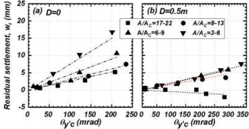
Figure 7 Normalized residual settlement vs. cumulative footing rotation of the footings grouped into different  $A/A_c$  ratios.
