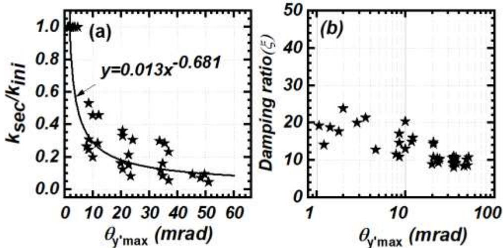
Figure 5. (a) Rotational stiffness degradation versus maximum footing rotation (b) damping ratio vs. footing rotation.
