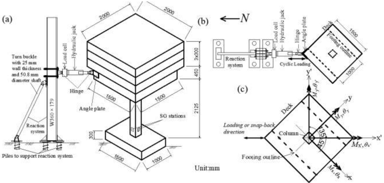
Figure 1 Schematic of the experimental model: (a) a semi-3D view, (b) top view, and (c) Definition of Cartesian coordinate system.
