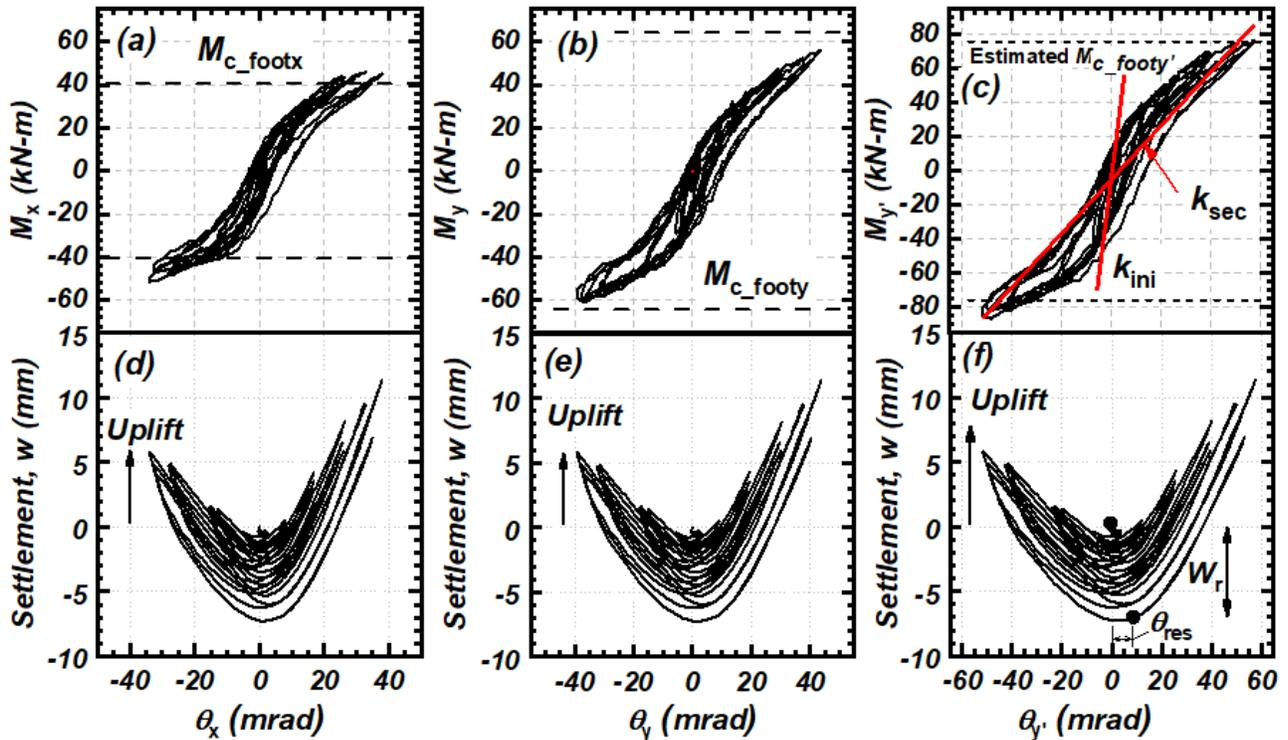
Figure 4. Results of test SE03 (a)  $M_x$  vs.  $\theta_y$  and  $w$  vs.  $\theta_y$  and (b)  $M_y$  vs.  $\theta_x$  and  $w$  vs.  $\theta_x$  and (c) resultant moment ( $M_R$ ) vs. rotation ( $\theta_R$ ) and settlement ( $w$ ) vs. rotation ( $\theta_R$ ) for test OE03.
