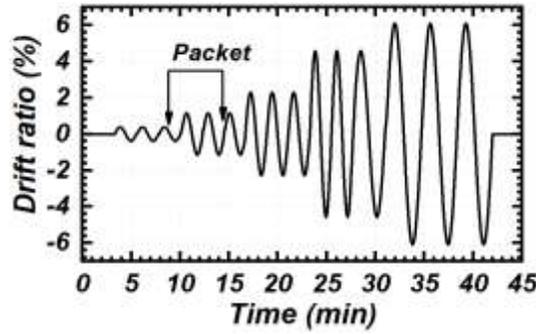
Figure 3. Typical time history of the drift under cyclic load.
